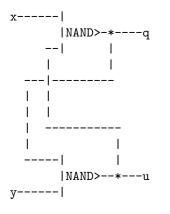
The inputs to this circuit are x and y, and the outputs are q and u. There are loops in this circuit – if we trace the output wire of the first NAND gate around to the input of the second NAND gate, to the output of the second NAND gate, to the input of the first NAND gate, to the output of the first NAND gate, we are back where we started: a loop. Thus, this circuit is sequential.
