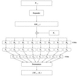
Figure 4.5: The DES Function  $f(R_{i-1}, K_i)$ .
