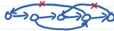
can remove 2 edges to make acyclic; removing only 1 always leaves a cycle
