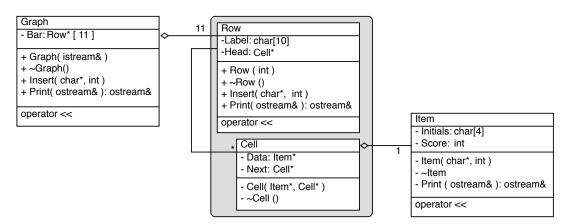
Figure 8.4: UML class diagram for Bargraph program.
