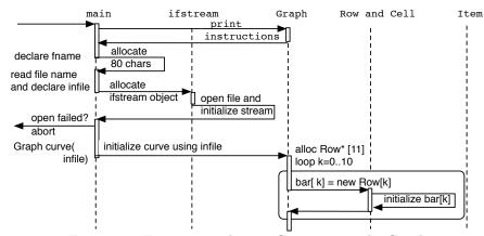
Figure 8.5: Event trace phase 1–Constructing the Graph.
