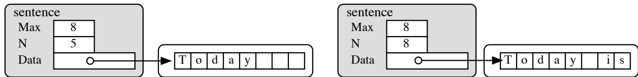
Figure 9.2: A FlexChars object after first growth spurt (left) and ready for second (right).
